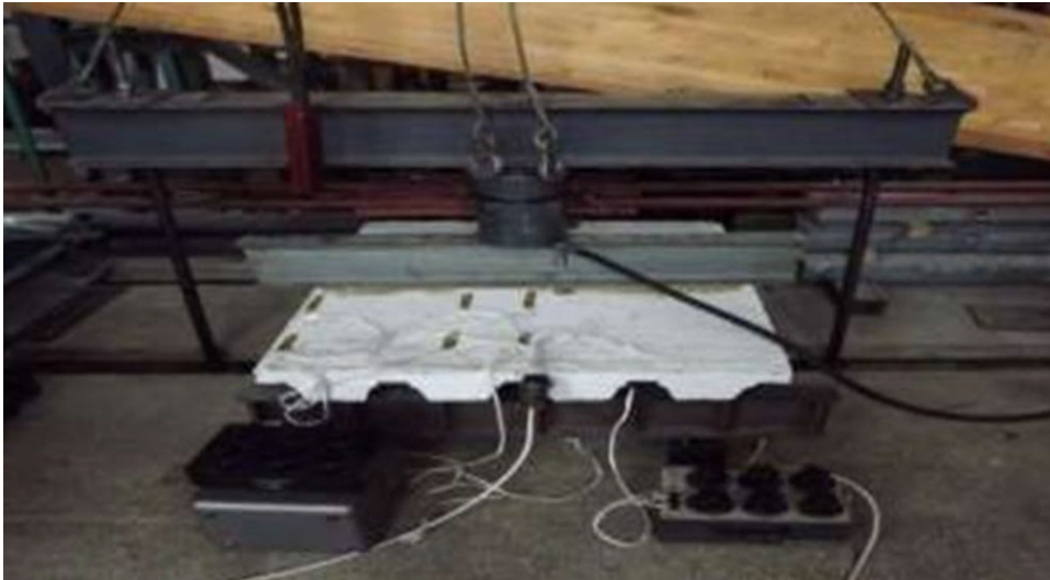
Figure 3 Placement of electric resistance strain gauges.
