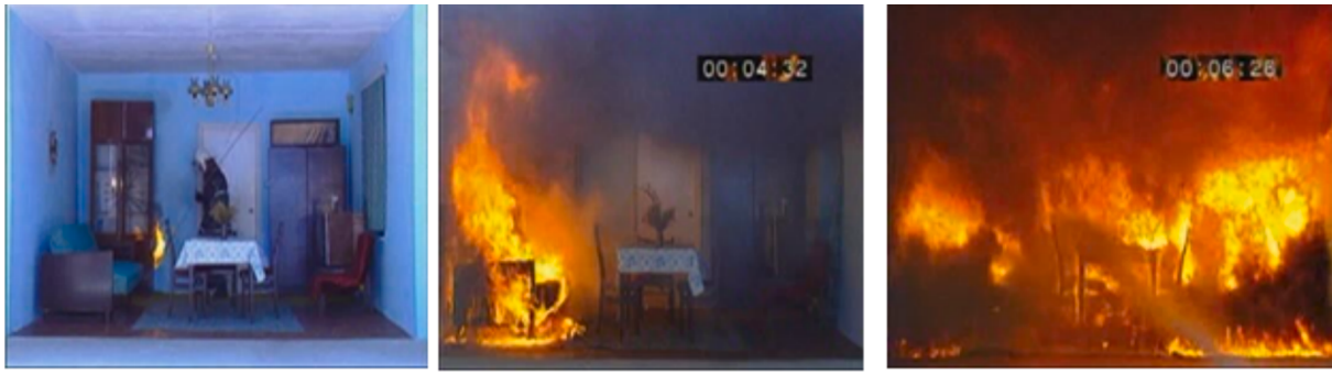
Fig. 18. Stages of arson and fire development of the room.
